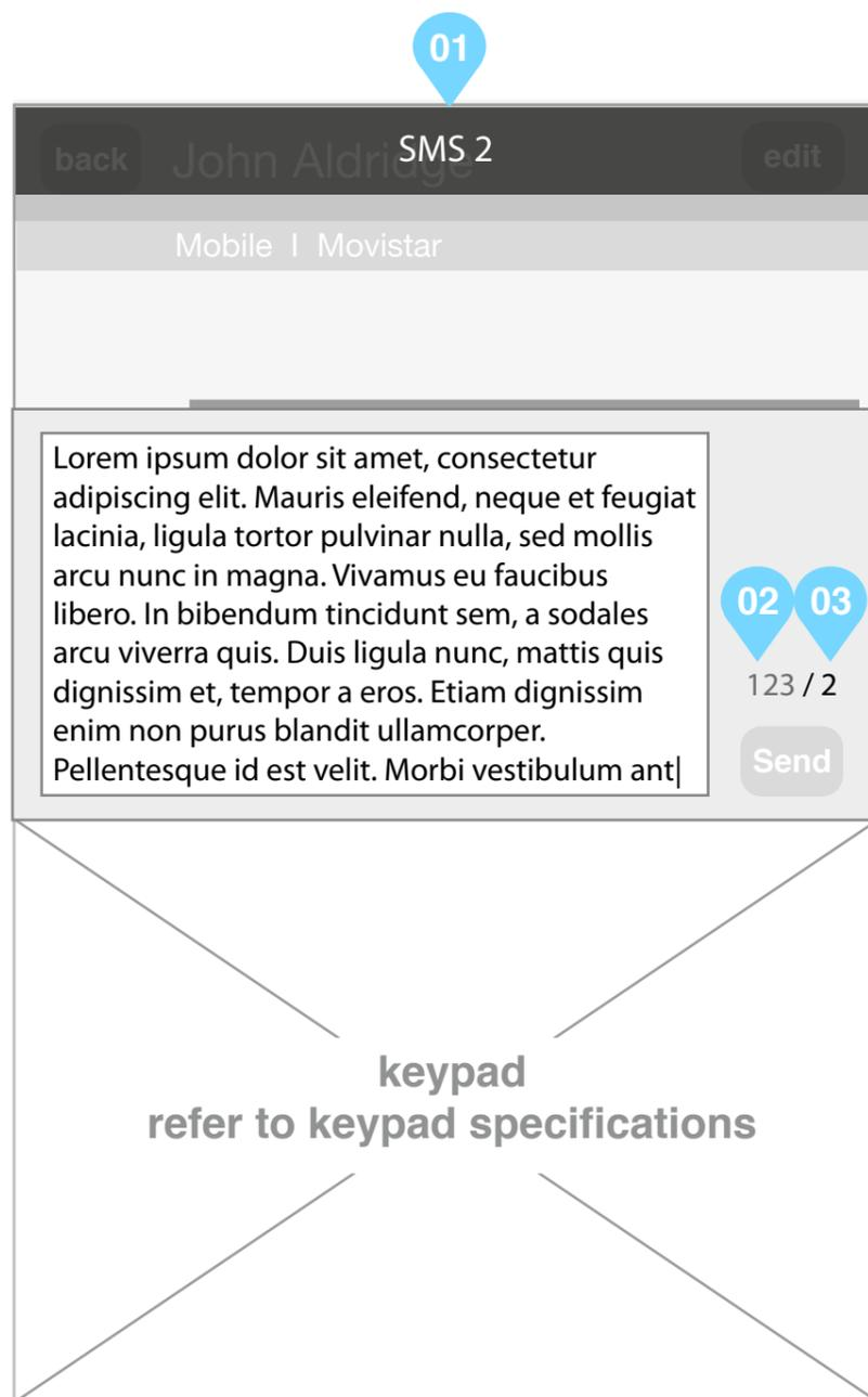
Wireframe illustrating the composing of an SMS message when the message to be sent comprises of multiple SMS packets
